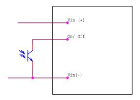
On/Off Circuit for positive or negative logic
